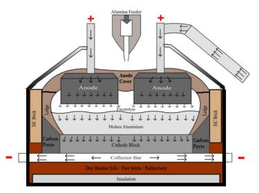
Figure 1. Cross-sectional view of Hall-Héroult cell.
